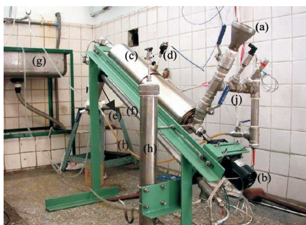
(a) Feed hopper; (b) auger motor; (c) reactor casing; (d) heating units and thermocouple connection; (e) ash tube; (f) condenser; (g) cooling water supply; (h) liquid-gas separator; (i) flue gas tubing; and (j) steam generator.
