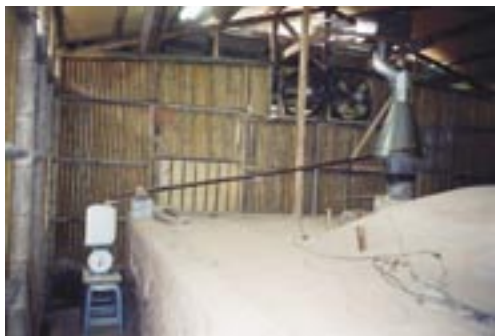
Fig. 4. Bamboo vinegar collection apparatus when the temperature of the chimney was < 150°C.
