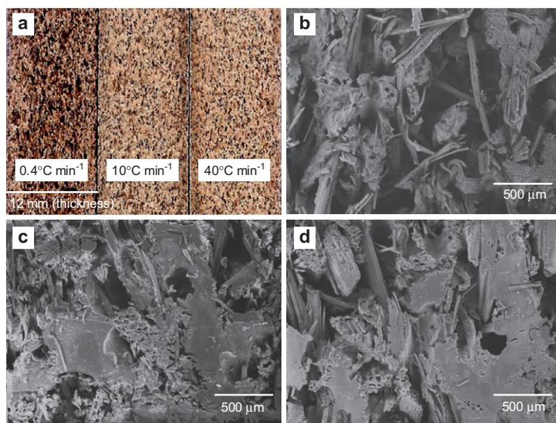
**Figure 3** Surface images (a) and SEM micrographs of BPC<sub>PLA</sub>s processed at cooling rates of 0.4 (b), 10 (c) and 40°C min<sup>-1</sup> (d).
