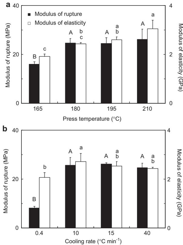
**Figure 1** Effects of press temperature (a) and cooling rate (b) on the modulus of rupture (MOR) and modulus of elasticity (MOE) of the BPC<sub>PLA</sub>s. Values are means $\pm$ SD ( $n=5$ ). Bars with different capital and lowercase letters indicate significant differences in the MOR and MOE values, respectively ( $P<0.05$ ).
