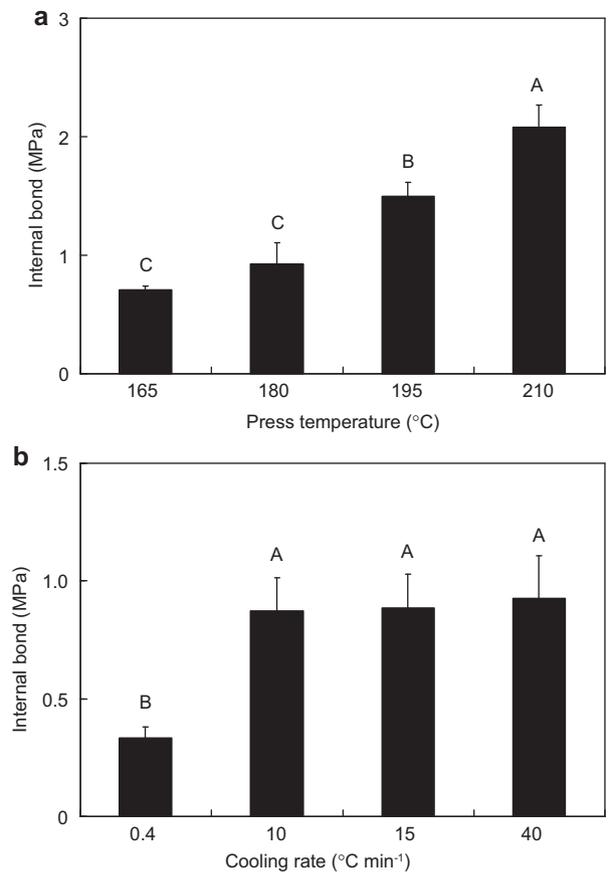
**Figure 2** Effects of press temperature (a) and cooling rate (b) on the internal bond (IB) of BPC<sub>PLA</sub>s. Values are means $\pm$ SD ( $n=5$ ). Bars with different capital letters indicate significant differences ( $P<0.05$ ).
