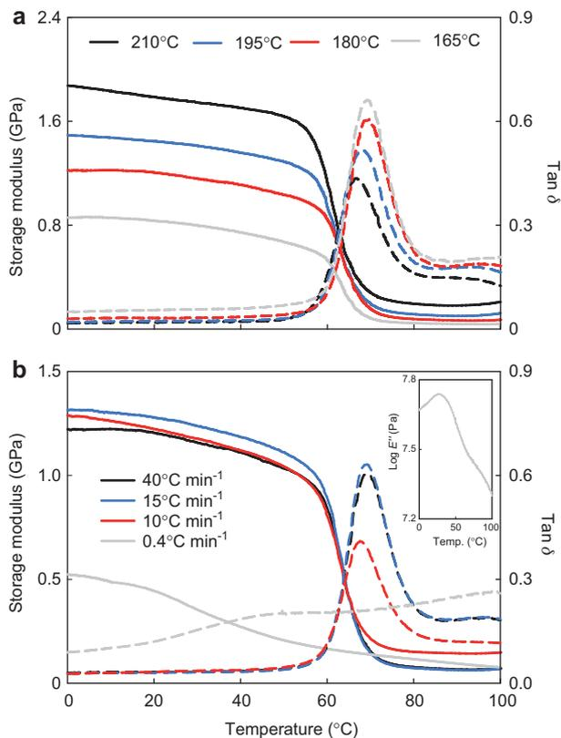
**Figure 4** Data calculated from dynamic mechanical measurements (DMA). Effects of press temperature (a) and cooling rate (b) on the storage modulus (solid line) and  $\tan \delta$  (dotted line) of BPC<sub>PLA</sub>S.
