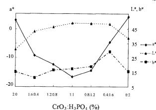
Fig. 2. Influence of  $CrO_3/H_3PO_4$  ratios in CP on the color of ma bamboo
