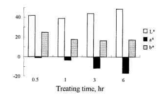
Fig. 3. Color changes of ma bamboo as a function of CP treating time
