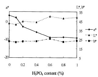
Fig. 1. Influence of H<sub>3</sub>PO<sub>4</sub> content in CCP on the color of ma bamboo
